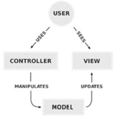
Figure 1 – MVC Architecture
