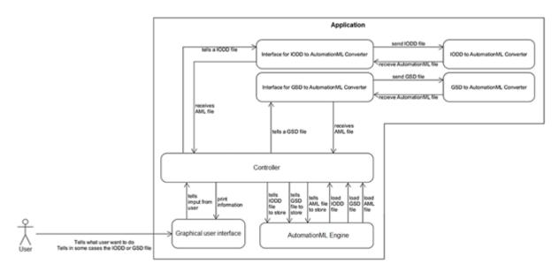
Figure 2 - Logic of the plugin
